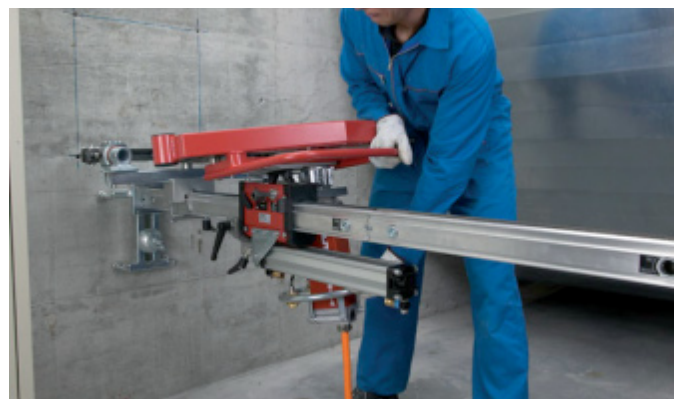
Guide the clamping piece into the slot in the carriage.
