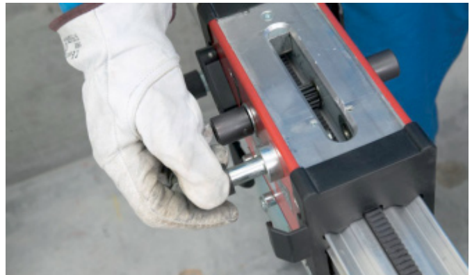
Pull out the carriage clamping pins.
