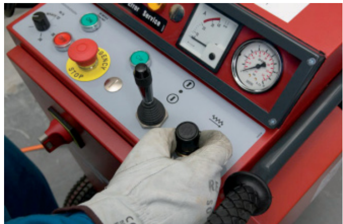
Set the advance pressure (DS WS10-E).
