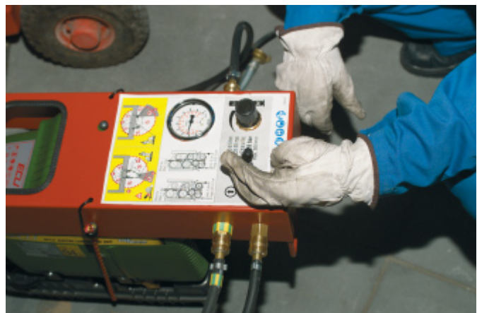
Operate the advance control valve (DS WS10).
