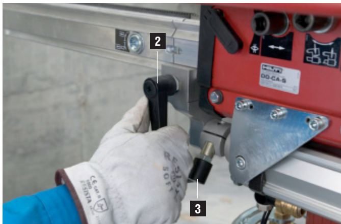
2 Piston rod securing lever
