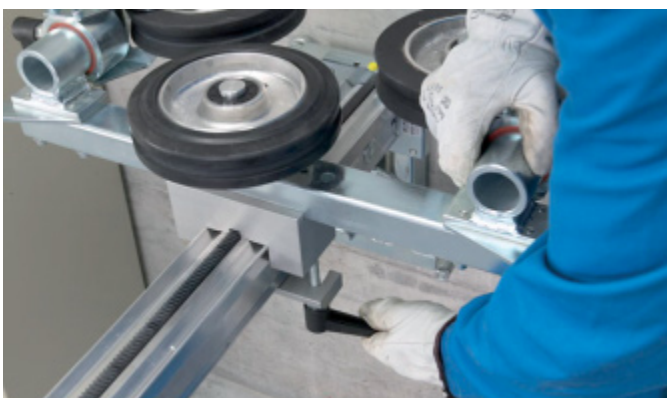
Close the locking bar and tighten the clamping lever.
