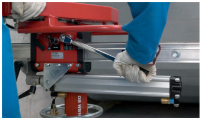
Push in the clamping pins and tighten them in a clockwise direction. Fit the end stop.
