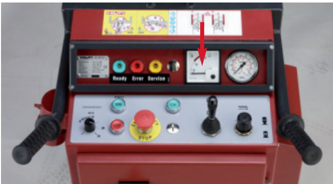
10.18 Current input is too high when idling and sawing (DS WS10-E)
