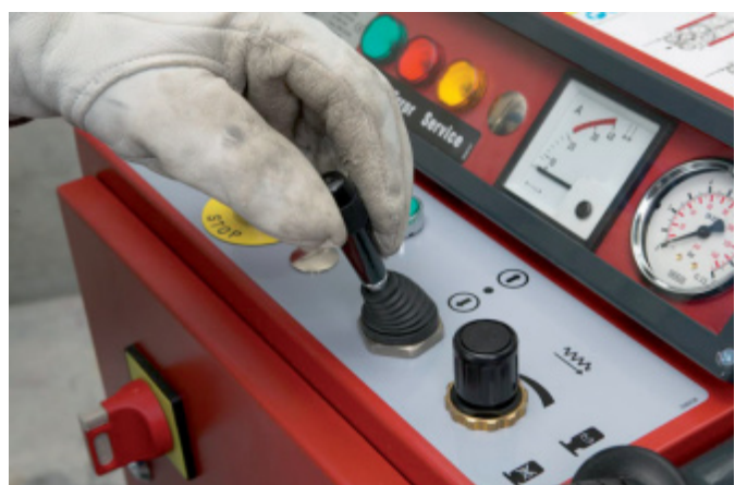
Operate the advance control valve (DS WS10-E).
