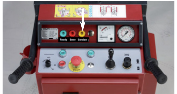
10.19 The service indicator lights and the drive unit may be inoperative
