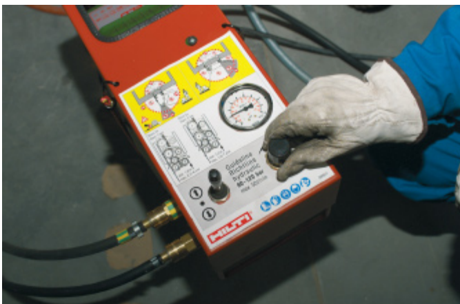
Set the advance pressure (DS WS10).
